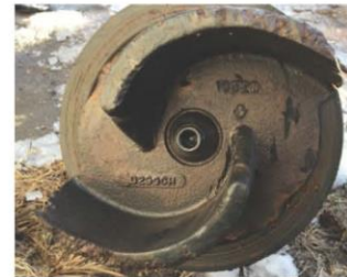
Severe wipe blockages may lead to service line replacement
